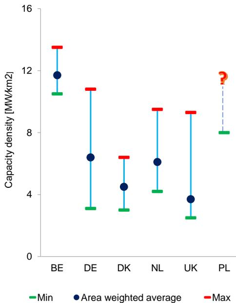
**Figure 2 – Mean and range of wind farm capacity density per market**
