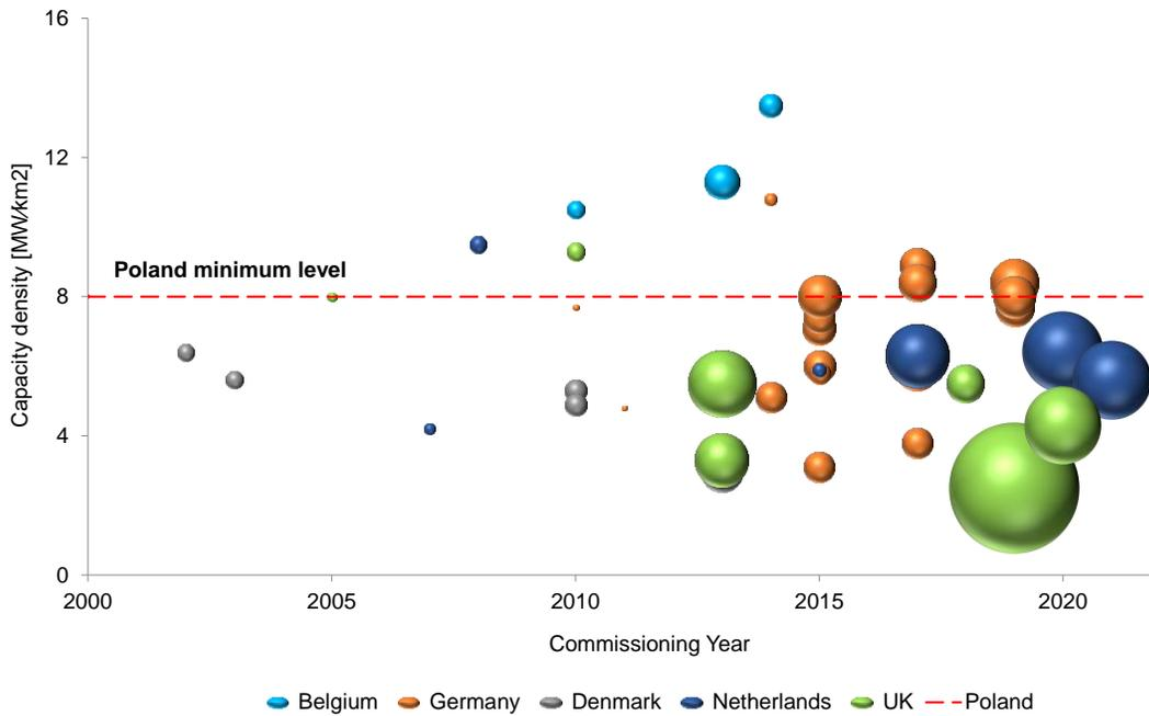
**Figure 1 – Offshore wind farm capacity density by country, size and maturity. A sample of projects representative of each market has been used for the plot. Each sphere refers to a project, and the size of the spheres depicts the size of the project as installed capacity (MW).**
