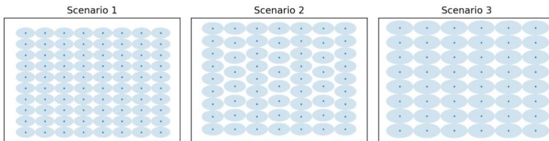
**Figure 4 – Layout scenarios considered. Ellipses illustrate the 7D by 4D turbine spacing assumed.**
