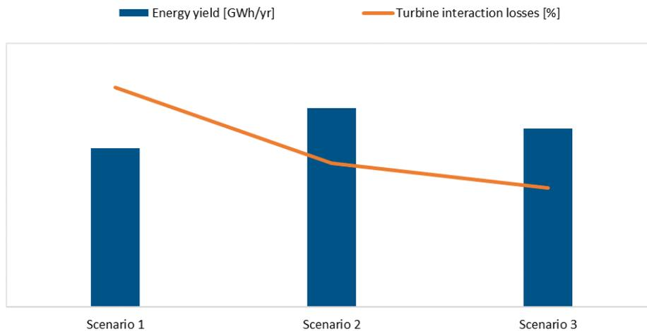
**Figure 5 – Indicative energy yield production (after turbine interaction effects) and turbine interaction effect losses estimated for the three scenarios considered.**
