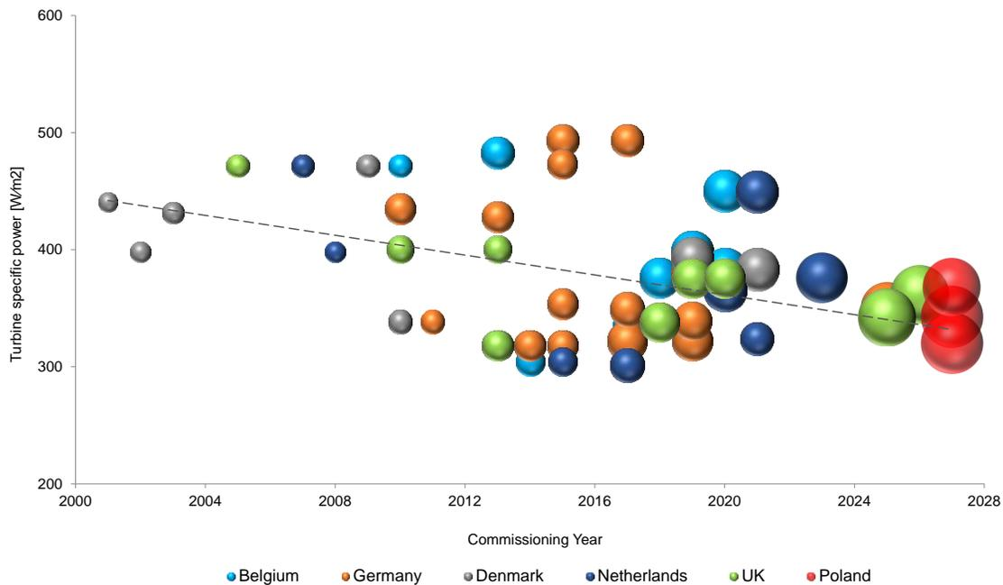
**Figure 3 – Trend of turbine specific power observed in Europe from 2000. Each sphere refers to a turbine model, and the size of the spheres depicts the rotor diameter.**
